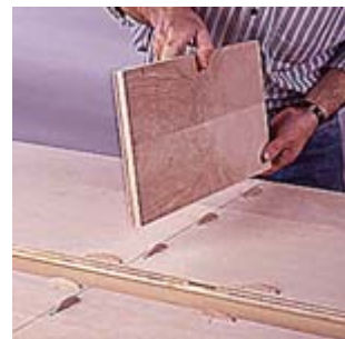
11--Install the plates and position the partitions followed by the backs. Finally, place the top panel in position.
