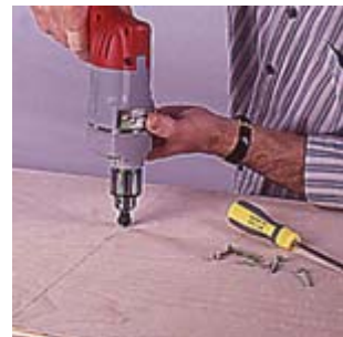
12--With all parts aligned, bore screwholes through the top and secure the panel. Turn the assembly over and fasten the bottom.
