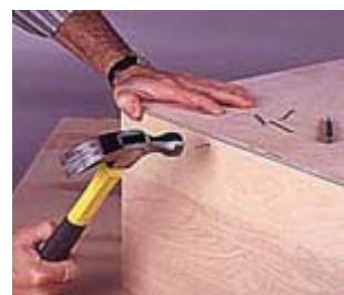
13--Use 6d finish nails in place of clamps to hold the ends tightly in place while the glue on the joining plates
