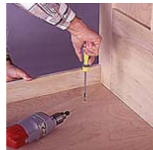
19--Place the platform assembly on the storage unit and tight against the headboard. Secure the platform with screws.
